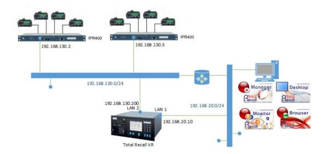
As we are recording in active mode, it is necessary to assign a valid static IP address to the LAN 2 interface of the Total Recall VR so that the Total Recall VR can receive RoIP traffic from the rest of the equipment on the network.
