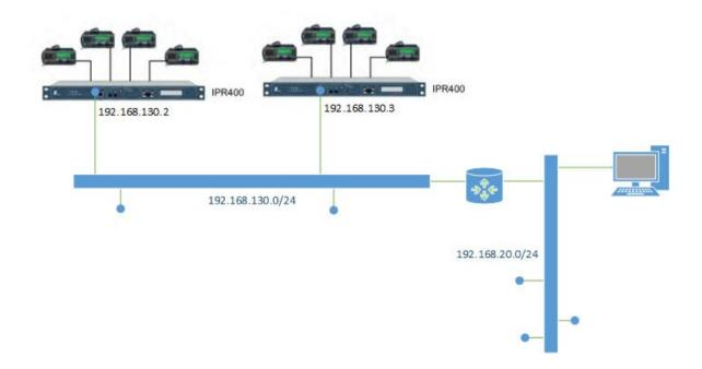
In addition we assume that the IPRs are on a separate network (as it is a good practice to separate RoIP traffic from the enterprise data traffic).
