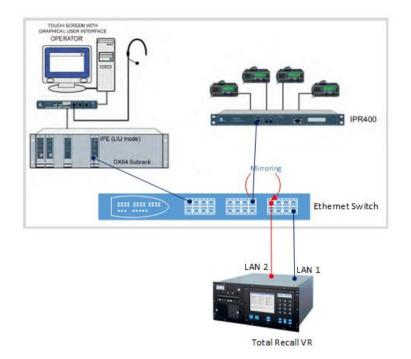
Note that we also connect the LAN 1 port of the Total Recall VR to the same switch. This allows us to add the Total Recall VR to the network and use Total Recall VR PC applications to access the Total Recall VR remotely via the LAN 1 interface while the LAN 2 interface is used to record radio communication.
