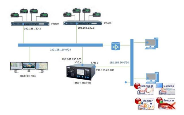
As we are recording in active mode, it is necessary to assign a valid static IP address to the LAN 2 interface of the Total Recall VR so that the Total Recall VR can receive RoIP traffic from the rest of the equipment on the network.
