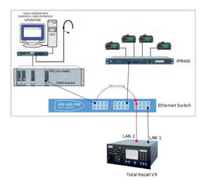
As we are recording in passive mode, we are using an Ethernet switch with SPAN port capability. The switch must be configured to SPAN the port connected to the IPE card to the port connected to the LAN 2 interface on the Total Recall VR.
