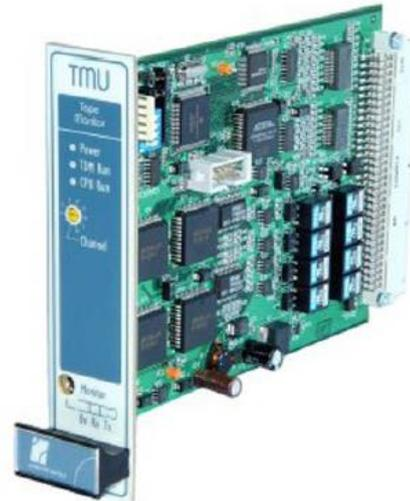
Each TMU provides 8 analogue feeds via two RJ45 connectors located on the backplane of the DX-Altus Server sub-rack as shown on the subsequent figure:
