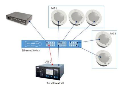
Note that we simply connect both LAN interfaces on the Total Recall VR to the same switch. The assumption here is that when a multicast packet arrives on one port of the switch, the switch simply copies the packet to all other active ports. As a result, all multicast packets will be present on the LAN 2 interface of the Total Recall VR.
