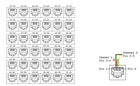
Note that recording channel numbering start from left on the top row and continues to right and down as shown on the previous image.
