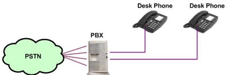
Figure 2: Analogue Telephone Connections (before)
