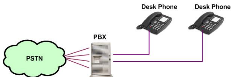
Figure 2: Analogue Telephone Connections (before)
