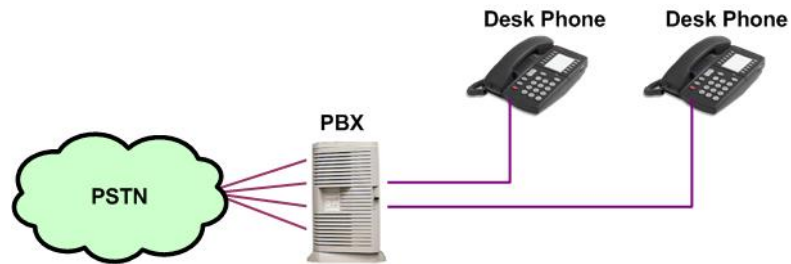
Figure 3: Analogue Telephone Connections (before)
