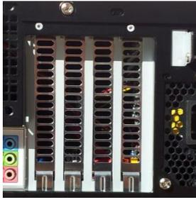
If your Total Recall VR has only VoIP recording channels, then blanking plates are fitted to all expansion slots. Total Recall VR does not need additional hardware to record VoIP calls.
