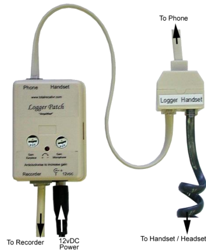
Figure 37: Logger Patch Wiring - Non-Standard Headset
