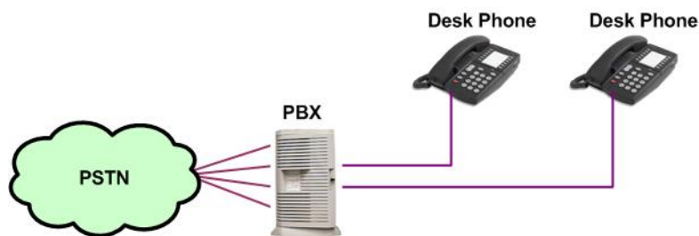
Figure 2: Analogue Telephone Connections (before)
