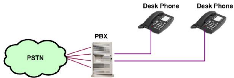
Figure 3: Analogue Telephone Connections (before)
