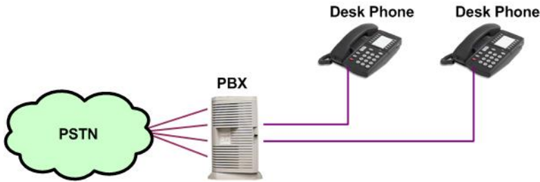
Figure 3: Analogue Telephone Connections (before)
