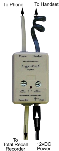
Figure 36: Logger Patch Wiring - Standard Headset
