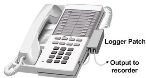
Figure 35: Digital Desk Phone with Logger Patch
