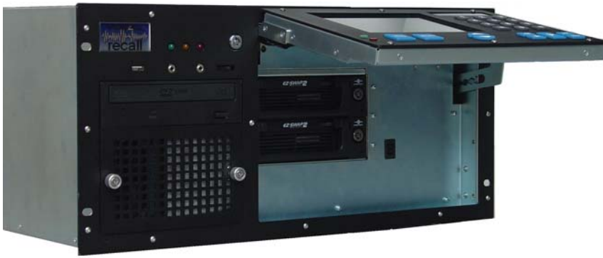
Tilting Colour LCD Control Panel, with swappable mirrored hard drives
